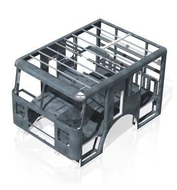
This remarkable cab begins with a Seagrave exclusive – a substantial three inch rectangular-tube steel subframe. Welded over this subframe is a completely enclosed, all-stainless steel superstructure that creates a protective cage. The entire structure is then covered with heavy gauge, stainless steel. The finished Capitol is one of three premiere cab choices, designed to outperform in longevity, durability, and saftey.
